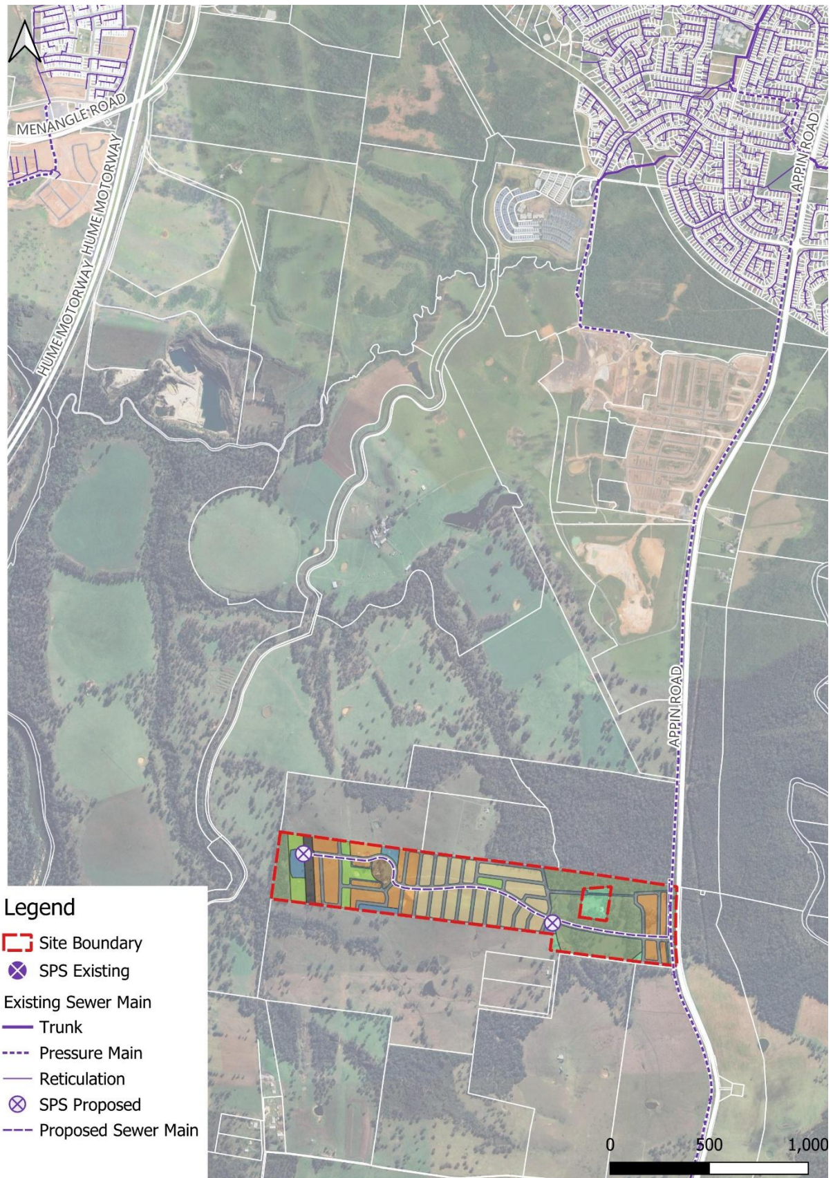
Figure 10 - Site Trunk Sewer Services
